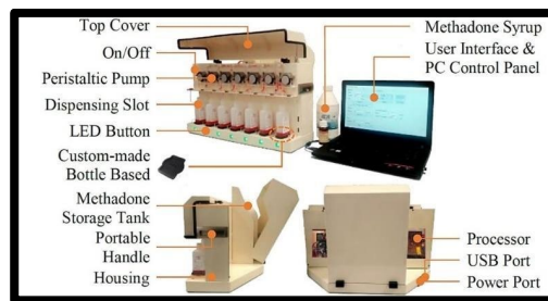
Figure 1: Isometric, side, and rear view of the automated methadone dispenser
